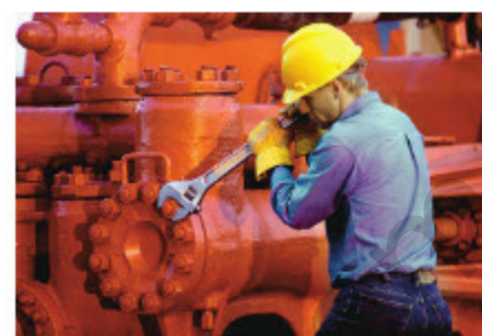
▲ The long handle of this wrench enables the user to produce a large torque without having to exert a very great force.
