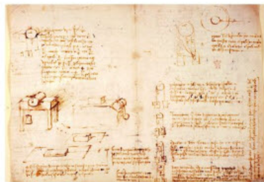
Sketches from the notebooks of Leonardo da Vinci showing experiments he performed on friction (Problem 74)
