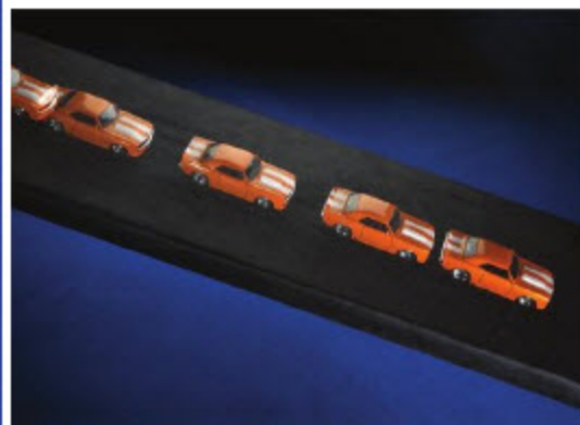
(a) Front wheels locked; rear wheels free to turn
