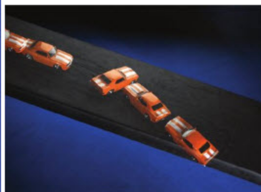
(b) Rear wheels locked; front wheels free to turn
