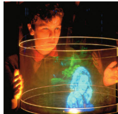
▲ A hologram creates a three-dimensional image in empty space. The image can be viewed from different angles to reveal different parts of the original subject.
