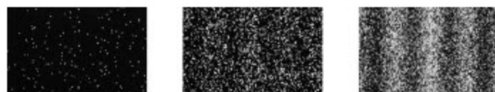
Two-slit diffraction pattern formed by electrons. This pattern appears even if the electrons pass through the device one by one.
