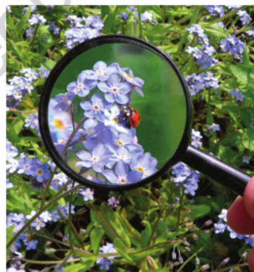
▲ A magnifying glass produces an enlarged image when held near an object. The image is upright and virtual.
