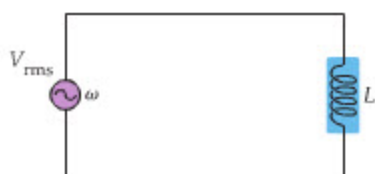
▲ FIGURE 24-13 An ac generator connected to an inductor
