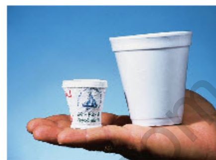
▲ Styrofoam has a very small bulk modulus, which means that even a relatively small increase in pressure can cause a large decrease in volume. The Styrofoam cup at left was immersed to a depth of 1955 m, where the water pressure is nearly 200 atm.
