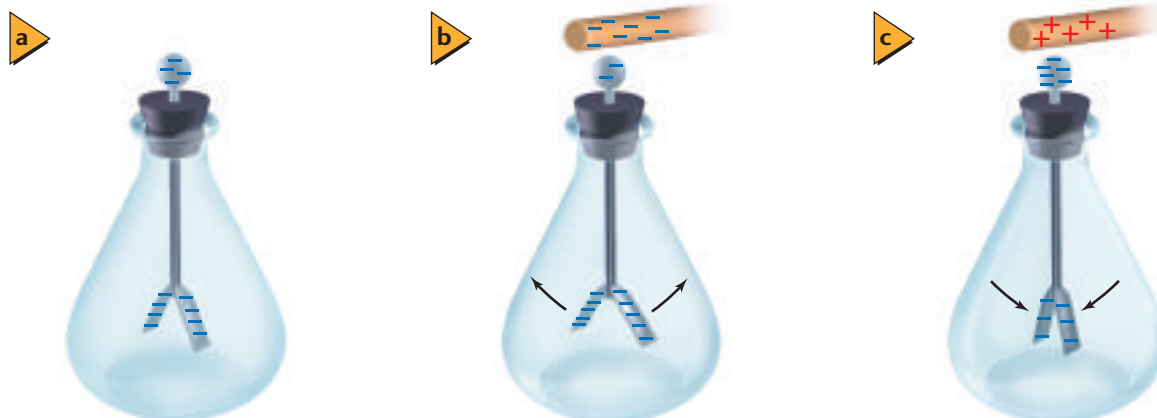
■ Figure 20-7 A negatively charged electroscope will have its leaves spread apart (a). A negatively charged rod pushes electrons down to the leaves, causing them to spread farther apart (b). A positively charged rod attracts some of the electrons, causing the leaves to spread apart less (c).
