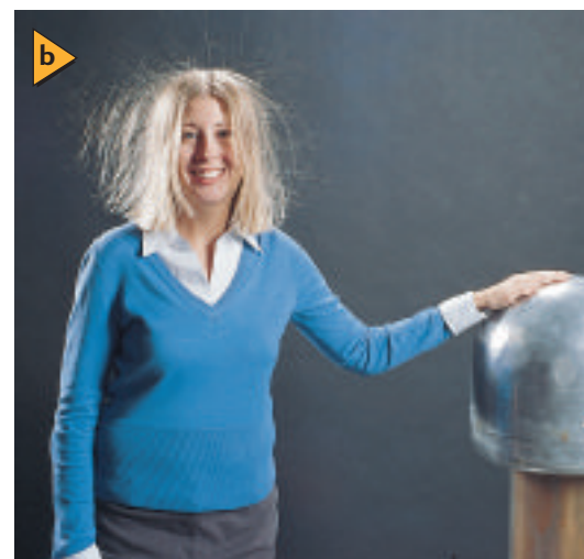
■ Figure 21-3 In the Van de Graaff generator (a) , charge is transferred onto a moving belt at A, and from the belt to the metal dome at B. An electric motor does the work needed to increase the electric potential energy. When a person touches a Van de Graaff generator, the results can be dramatic (b) .
