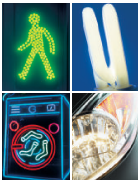
Clockwise from the upper left, the photos show LEDs, a fluorescent light, a halogen light, and gas-discharge lamps in the form of neon lights.
