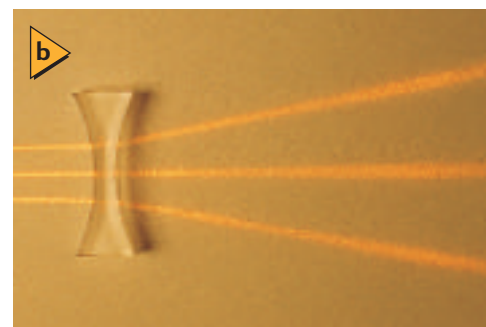
■ Figure 18-9 A convex lens causes rays of light to converge (a) . A concave lens causes rays of light to diverge (b) .
