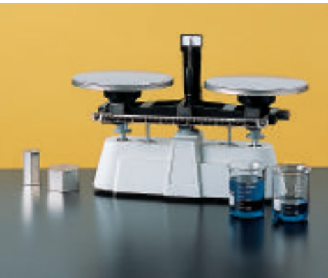
■ Figure 7-14 The platform balance shown here allows you to measure the force on a mass due to Earth's gravity.
