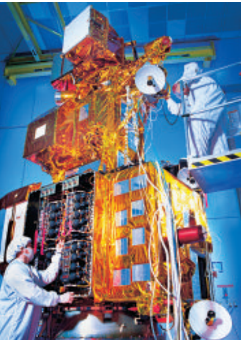
■ Figure 7-10 Landsat 7 , a remote sensing satellite, has a mass of about 2200 kg and orbits Earth at an altitude of about 705 km.
