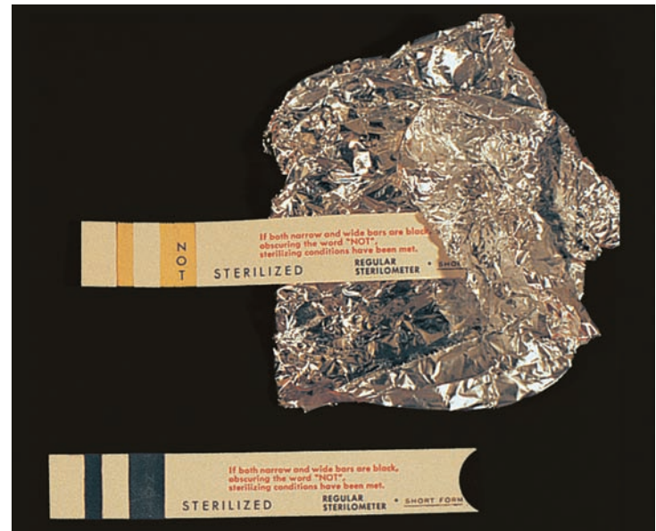
Figure 7.3 Examples of sterilization indicators. The strips indicate whether the item has been properly sterilized. The word NOT appears if heating has been inadequate. In the illustration, the indicator that was wrapped with aluminum foil was not sterilized because steam couldn't penetrate the foil.
