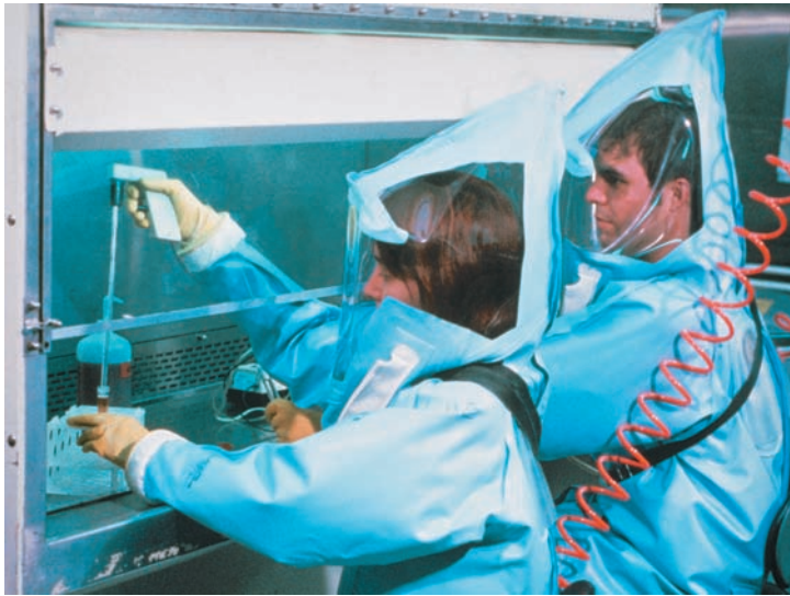
Figure 6.8 Technicians in a biosafety level 4 (BSL-4) laboratory. Personnel working in a BSL-4 facility wear a “space suit” that is connected to an outside air supply.
