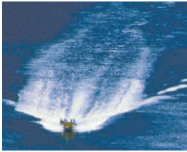
Figure 9.15 The large bow wave is the result of the boat moving faster than the speed of the waves in water.
