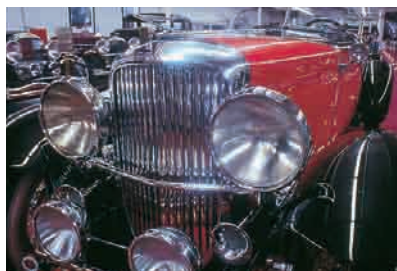
Figure 10.17 The reflectors used in solar cookers and headlights are deliberately designed so that they do not have a perfectly parabolic shape.
