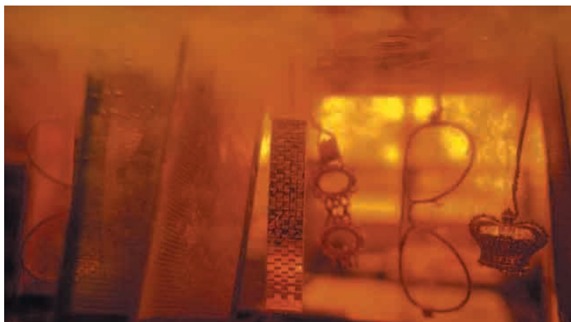
Figure 13.8 A less expensive metal can be silver-plated to produce an attractive and corrosion-resistant surface. The object to be plated is connected to a circuit as the cathode. It is suspended in a solution containing silver cyanide. The silver ions are attracted to the cathode, where they combine with electrons and become solid silver atoms that remain permanently attached to the surface of the cathode.
