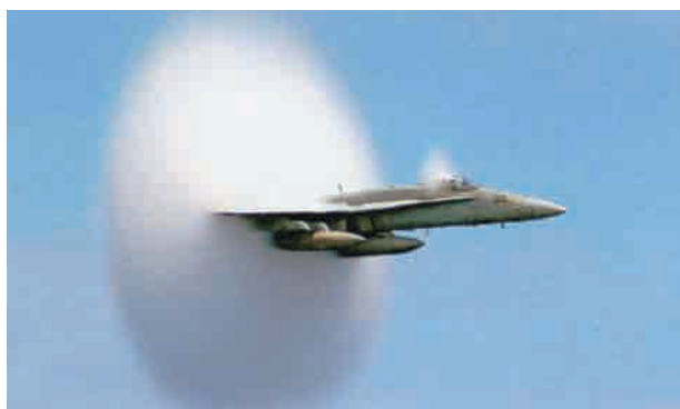
Figure 9.13 The shock wave as a jet breaks the sound barrier is visible because the increased pressure causes water vapour to condense.
