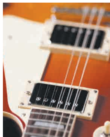
Figure 15.10 Electric guitar pickups rely on Lenz's law.
