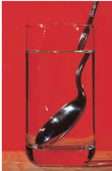
Figure 11.2 Light refracts, or bends, toward the normal when it passes from air into water or glass.
