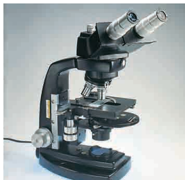
Figure 12.22 The lens arrangement of a microscope is similar to that of an astronomical telescope. In a binocular microscope, the light from the objective lens is split in two by prismatic mirrors and directed to the eyepiece lenses.
