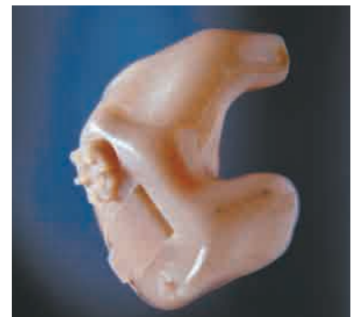
Figure 9.7 A hearing aid is composed of three distinct components: a microphone, an amplifier, and a speaker. Improvements in technology allow for higher quality components of smaller and smaller sizes. The amplifier often contains a programmable computer chip.
