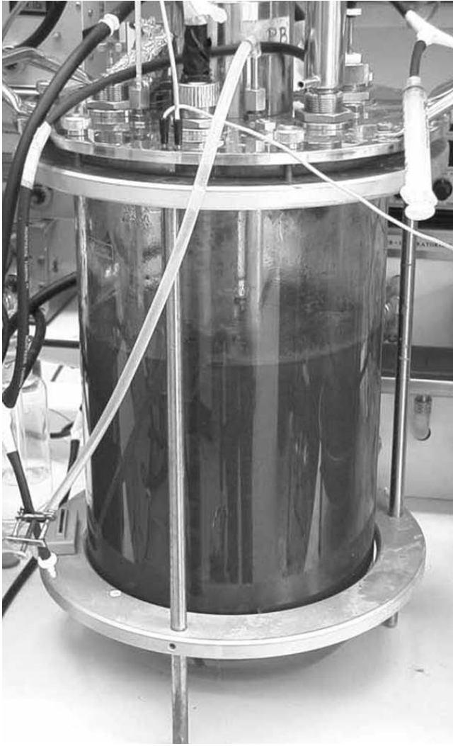
FIGURE 9.12 Bioreactor Containing Candidatus Brocadia anammoxidans , Anaerobic Bacterium That Can Degrade Ammonium Novel metabolic properties enable these anaerobes to degrade ammonium from wastewater in a single step.
