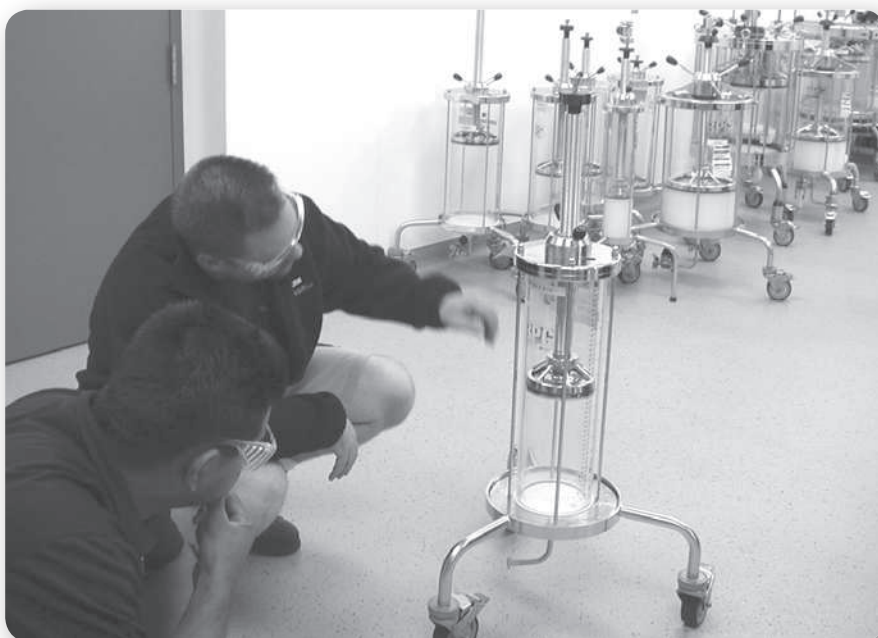
Lab Supervisor Preparing a Purification Column to Separate a Commercial Biological Product.
