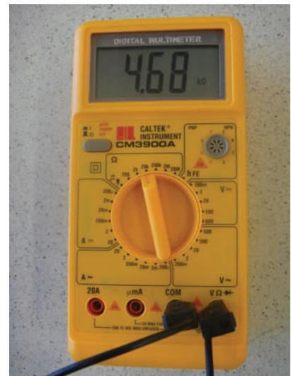
Figure 11.14 Digital multimeter measuring the resistance of a 4.7 kΩ resistor. The meter is set on the 20 kΩ range and so the resistance recorded is 4.68 kΩ.
