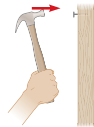
Figure 5.8 The moving hammer has kinetic energy and can do work on the nail, driving it into the wall.
