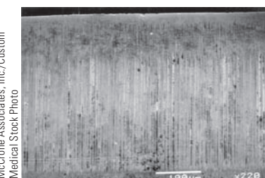
The edge of a razor blade looks smooth to the eye, but under a microscope proves to have numerous irregularities.
