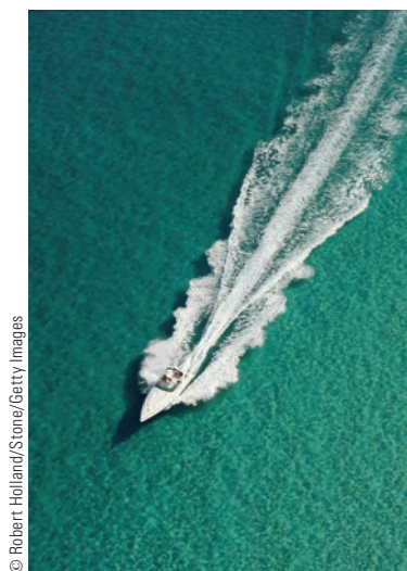
Figure 14.12 The V-shaped bow wave is formed because the boat travels at a speed greater than the speed of the water waves. A bow wave is analogous to a shock wave formed by a jet traveling faster than sound.
