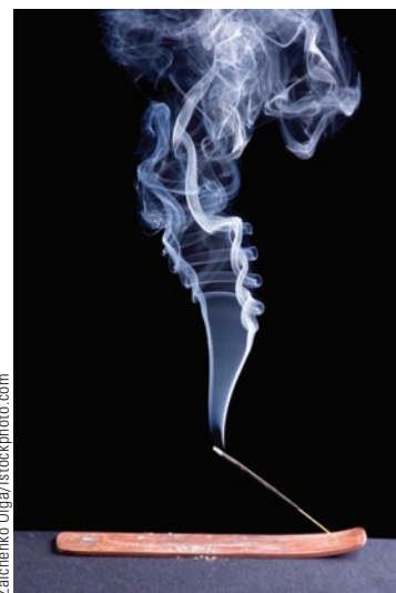
Figure 9.28 Hot gases made visible by smoke particles. The smoke first moves in laminar flow at the bottom and then in turbulent flow above.
