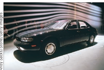
Figure 9.27 An illustration of streamline flow around an automobile in a test wind tunnel. The streamlines in the airflow are made visible by smoke particles.
