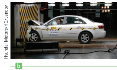
Figure 6.4 (Example 6.2) (a) This car's momentum changes as a result of its collision with the wall. (b) In a crash test (an inelastic collision), much of the car's initial kinetic energy is transformed into the energy it took to damage the vehicle.
