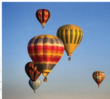
Hot-air balloons. Because hot air is less dense than cold air, there is a net upward force on the balloons.
