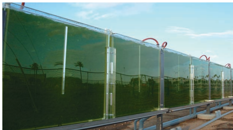
▲ Figure 10.3 Alternative fuels from algae. The power of sunlight can be tapped to generate a sustainable alternative to fossil fuels. Species of unicellular algae that are prolific producers of plant oils can be cultured in long, transparent tanks called photobioreactors, such as the one shown here at Arizona State University. A simple chemical process can yield “biodiesel,” which can be mixed with gasoline or used alone to power vehicles.
