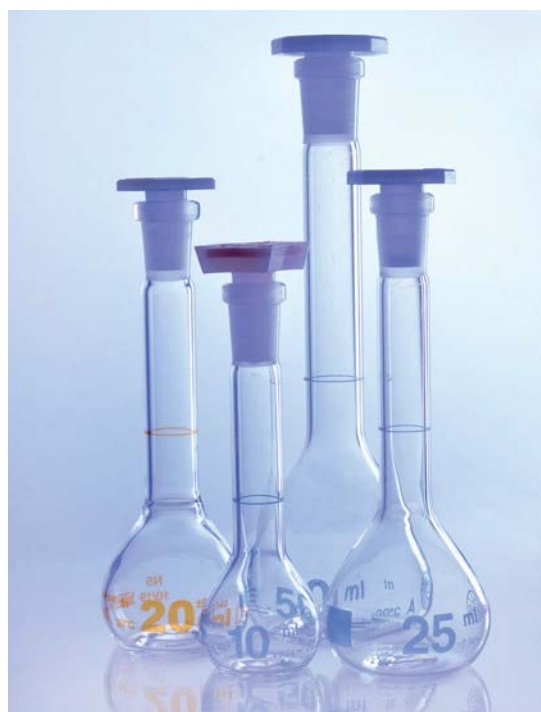
Figure P2.2 Volumetric flasks are used to make up standard solutions of known concentration accurately.
