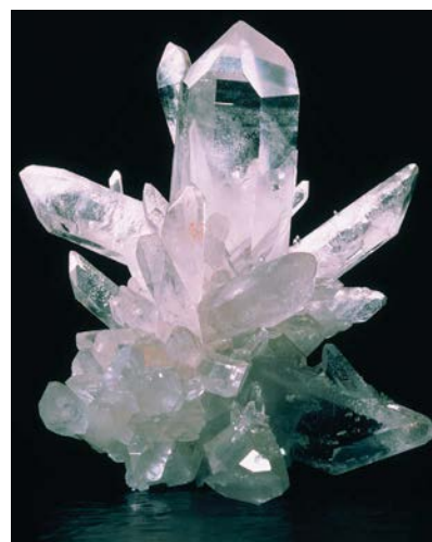
Figure 5.14 The shape of these quartz crystals reflects the regular arrangement of the silicon and oxygen atoms.
