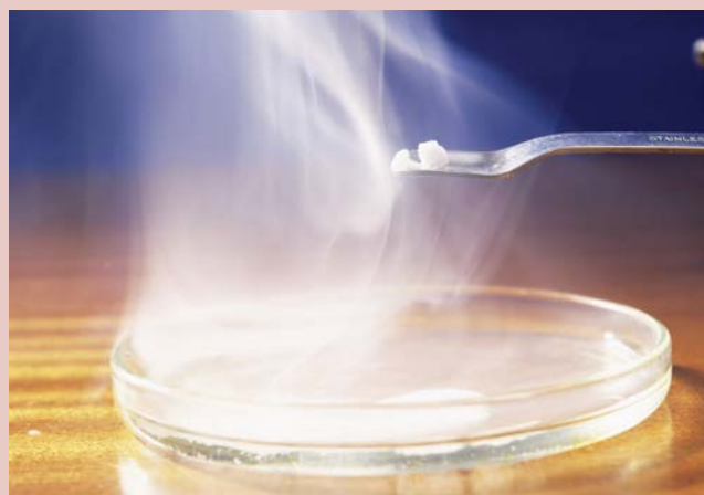
Figure 10.14 Solid phosphorus(V) chloride is hydrolysed in water, releasing white fumes of hydrogen chloride gas.
