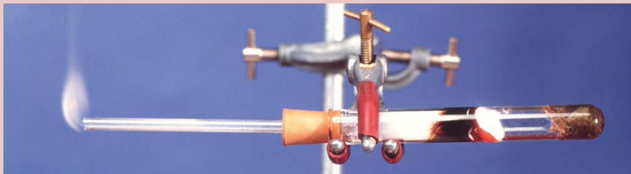
Figure 11.6 An experiment showing magnesium reacting with steam. The steam is given off from mineral wool soaked in water at the right-hand end of the test tube. The white magnesium oxide formed is visible inside the test tube and the hydrogen gas produced in the reaction has been ignited at the end of the straight tube.
