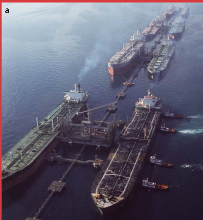
Figure 13.1 a Nitrogen gas is used in the hold of oil tankers above the crude oil as it is pumped ashore. This unreactive gas helps to prevent the chance of an explosive mixture of crude oil vapour and air forming inside the tanker. b Sulfur can be mined from underground deposits by pumping down super-heated water to melt the sulfur (it melts at about 115°C). The molten sulfur is then forced to the surface under pressure and allowed to solidify back into a brittle, yellow solid. The ‘crown-shaped’ sulfur molecules, S_8 , can pack together in regular patterns, forming crystals.
