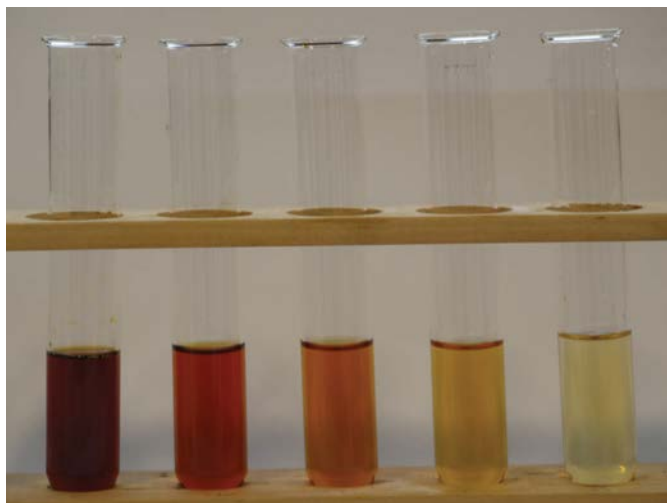
Figure 22.16 The rate of reaction between propanone and iodine can be followed by the loss of colour of the reaction mixture as the reaction proceeds.
