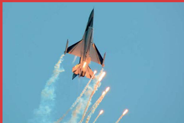
Figure 11.1 A military plane releasing its decoy flares to protect it from missile attack.
