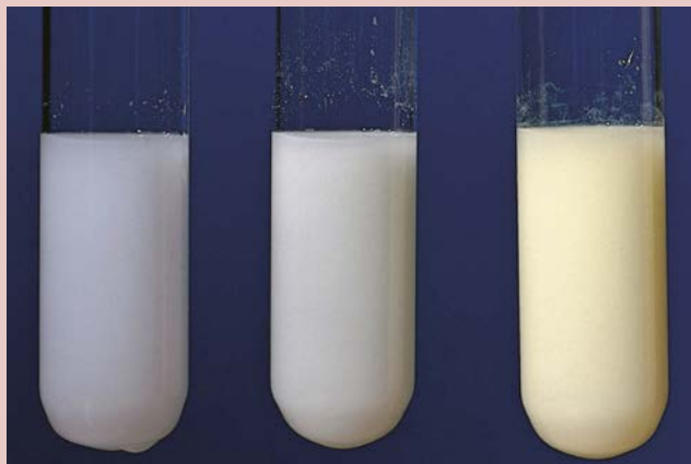
Figure 12.4 Colours of the silver halide precipitates: silver chloride (on the left), silver bromide and silver iodide (on the right).
