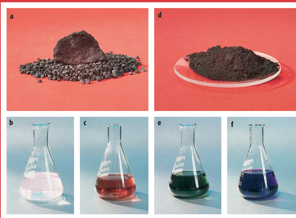
Figure 20.1 a manganese(0), the metal; b manganese(II) as \text{Mn}^{2+}(\text{aq}) ions; c manganese(III) as \text{Mn}^{3+}(\text{aq}) ions; d manganese(IV) as \text{MnO}_2 ; e Mn(VI) as \text{MnO}_4^{2-} as with parts b and c ions; f Mn(VII) as \text{MnO}_4^- as with parts b and c ions. Manganese metal is a good reductant, whereas \text{MnO}_4^-(\text{aq}) in acidic solution is a good oxidant.
