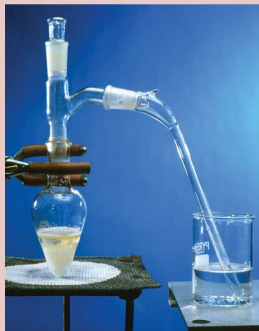
Figure 17.4 Bromoethane being distilled off following the reaction between ethanol and hydrogen bromide. The white solid visible in the pear-shaped flask is sodium bromide (as crystals). The sodium bromide reacts with concentrated sulfuric acid to make the hydrogen bromide needed for the reaction.
