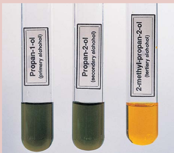
Figure 17.8 Before warming with the labelled alcohol, each of these tubes contained orange acidified potassium dichromate(VI) solution. After warming, the orange dichromate(VI) ions have been reduced to green chromium(III) ions by the primary and secondary alcohols. This shows that both the primary and secondary alcohols have been oxidised but the tertiary alcohol, 2-methylpropan-2-ol, has not.
