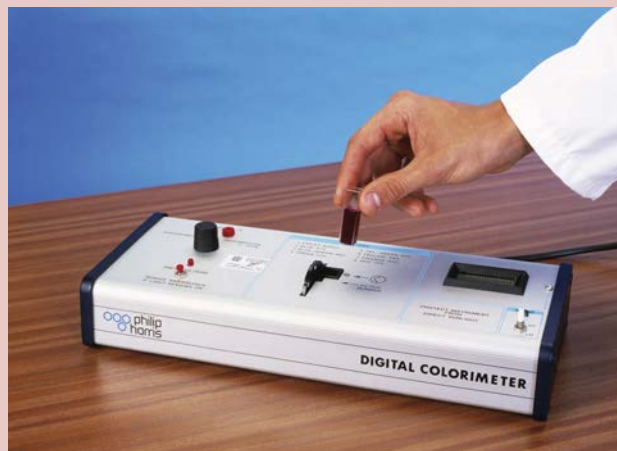
Figure 22.2 A colorimeter can be used to monitor the progress of a reaction. It measures the transmission of light through a 'cell' containing the reaction mixture. The less concentrated the colour of the reaction mixture, the more light is transmitted through the 'cell'.
