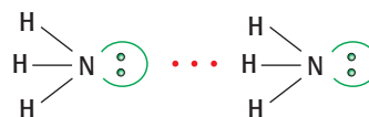
Figure 4.41 Hydrogen bonding between two ammonia molecules. A hydrogen bond is represented by a line of dots.
