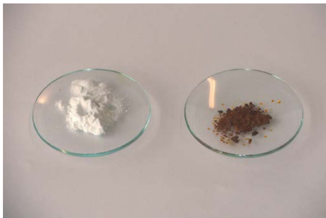
Figure 1.12 Iron(II) chloride (left) and iron(III) chloride (right). These two chlorides of iron both contain iron and chlorine, but they have different formulae.
