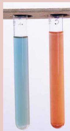
Figure 18.5 The 'before' and 'after' observations when Fehling's solution is warmed with an aldehyde, such as ethanal.
