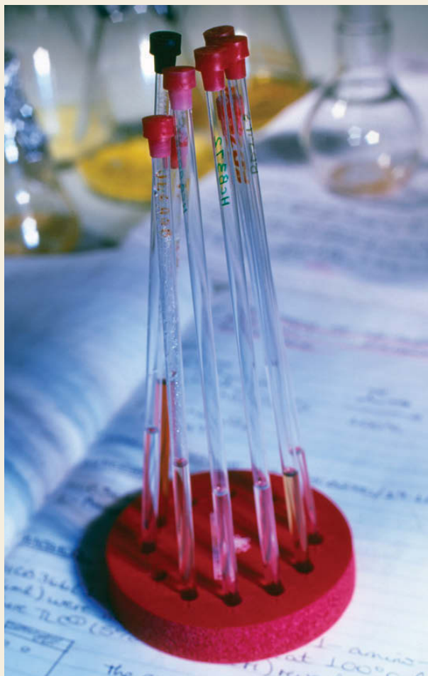
Figure 29.16 Samples dissolved in a solvent in narrow tubes ready for NMR analysis.
