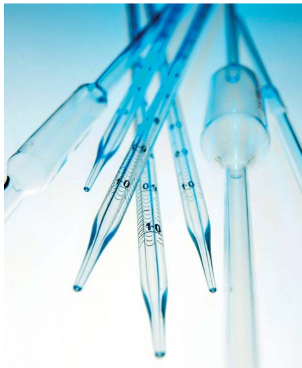
Figure P2.3 Volumetric and graduated pipettes are used to transfer accurate volumes of liquid. Volumetric pipettes give greater accuracy than graduated pipettes, due to the single line to measure to on the thin section above the bulge.
