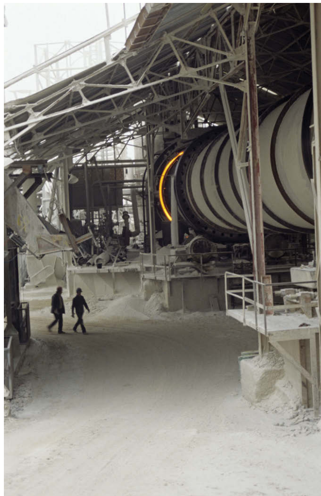
Figure 11.8 In a rotating lime kiln, calcium carbonate undergoes thermal decomposition to form calcium oxide and carbon dioxide.
