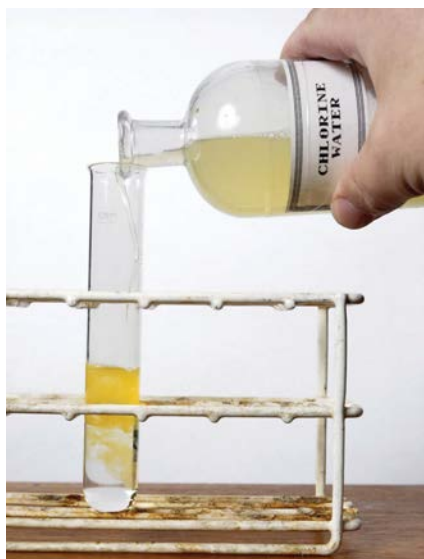
Figure 20.22 Aqueous chlorine displaces bromine from a solution of potassium bromide. We can use E^\ominus values to explain why a halogen higher in Group 17 displaces a halogen lower in the group from a solution of its halide ions.
