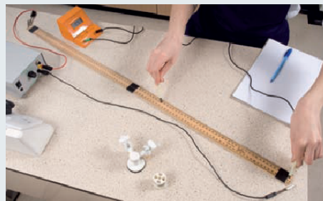
fig. 4.2.14 Set-up for variation of resistance investigation
