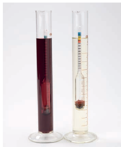
fig. 2.1.5 A hydrometer floats lower in the lower density (more alcoholic) red wine than in the white wine.
