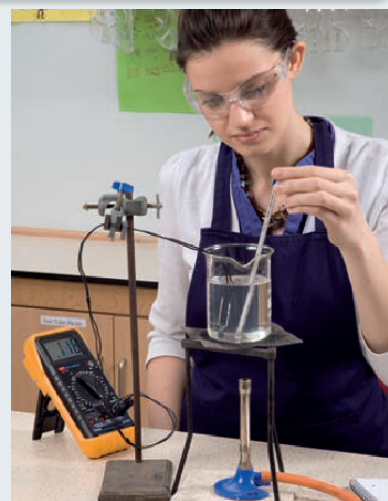
fig. 4.2.24 Calibrating a thermistor.
