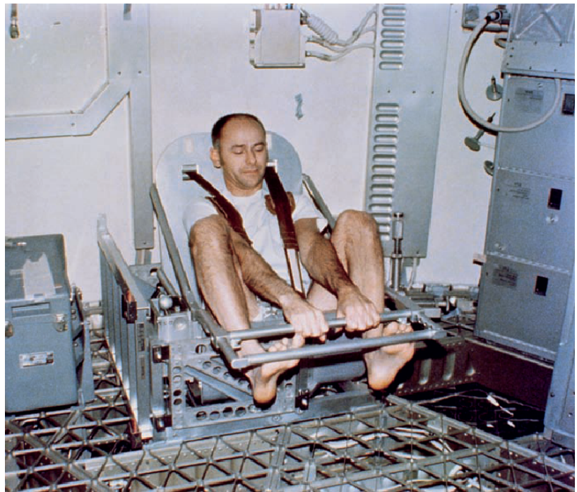
fig. 1.2.12 Newton's first law in action. It is important to know about changes in body mass happening to astronauts during long periods in orbit. Obviously bathroom scales are useless in this situation. This device uses the inertia of the astronaut's body to affect the way in which oscillations happen – the oscillations are then timed and used to calculate the mass of the astronaut.
