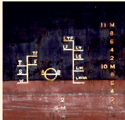
fig. 2.1.4 The Plimsoll Line on a ship indicates the safe loading level. The water surface must not be above the line indicating the temperature and location of the seas to be crossed (for example TF refers to tropical fresh water). As cargo is loaded, the ship will sink lower to displace a greater weight of water and thus balance the new, heavier overall weight of the ship.
