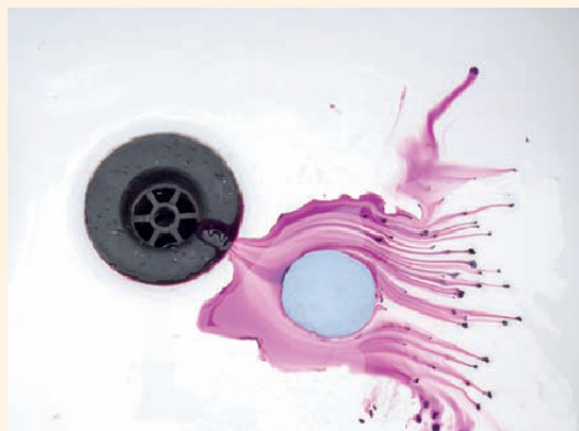
fig. 2.1.9 A few crystals of potassium manganate(VII) will produce purple trails in the water flow which can then be made to pass around objects made from Blu-tack®. You can alter the flow rate and the obstacle shapes in order to see how the flow changes.
