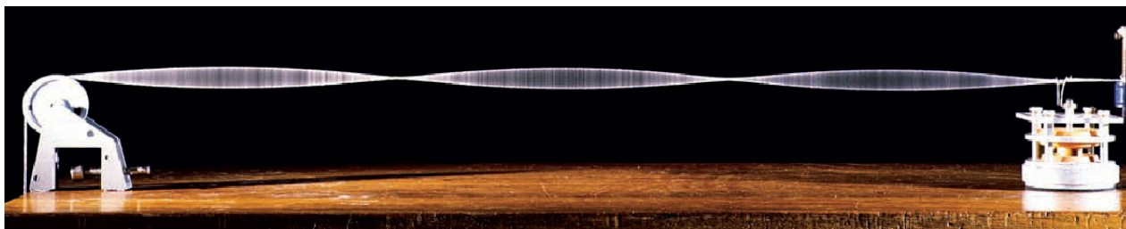
fig. 3.1.13 Standing wave on a vibrating string. A standing wave, also known as a stationary wave, is a wave that remains in a constant position. If the medium (here the string) is not moving with respect to the wave, then the standing wave is a result of interference between two waves travelling in opposite directions, in this case waves reflecting from either end of the string.
