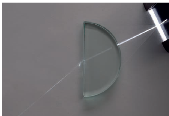
fig. 3.2.7 Investigating total internal reflection.
