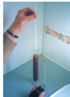
fig. 2.2.18 Chocolate falling-ball viscometer.
