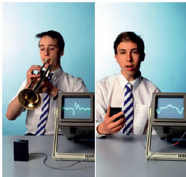
fig. 3.1.22 Oscilloscope traces of vibrations from a singer's vocal cords and a trumpet.
