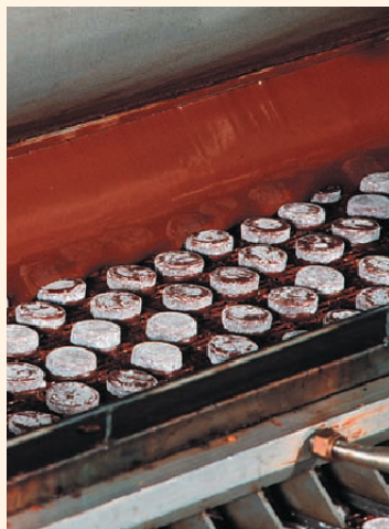
fig. 2.2.16 The enrobing process.
