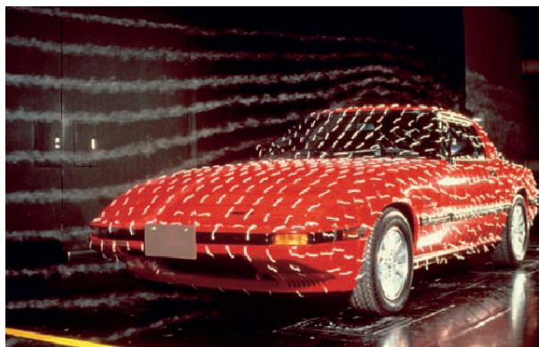
fig. 2.1.8 Smoke streamlines show laminar flow of air over a well-designed car.
