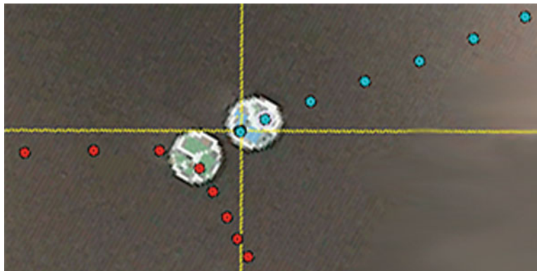
FIGURE 7-14 ■ A video analysis of a collision between two pucks. A puck traveling on an air table hits another stationary puck with a glancing blow. They both travel off in different velocities in such a way that momentum is conserved.
