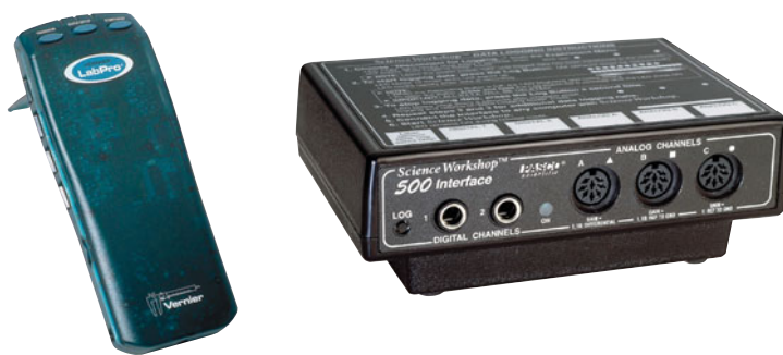
FIGURE 1-11 ■ Two electronic interfaces used in popular introductory physics computer data acquisition systems: The LabPro Interface (Vernier Software and Technology) and the Science Workshop 500 Interface (PASCO scientific).
