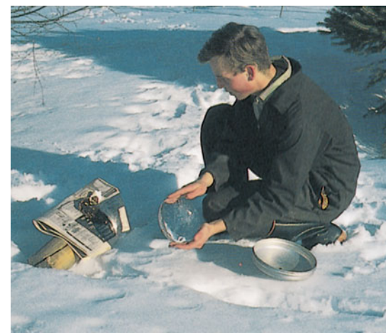
A fire is being started by focusing sunlight onto newspaper by means of a converging lens made of clear ice. The lens was made by freezing water in the shallow vessel (which has a curved bottom).
