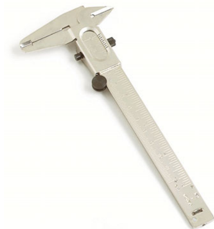
FIGURE 1-8 ■ Vernier calipers are cleverly designed to make length measurements to within 1/10 of a millimeter.
