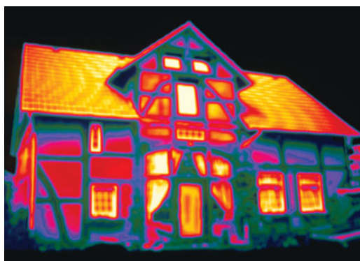
FIGURE 19-27 ■ Thermogram of a house showing the distribution of heat over its surface. The color coding ranges from white to yellow for the warmest areas (greatest heat loss from windows, etc) through red to purple and green for the coolest areas (greatest insulation). This thermogram shows that the roof and windows (yellow) are poorly insulated, while the walls (red, purple, and green) are losing the least heat. Thermograms are often used to check houses for heat loss, so that they can be made more energy efficient through improved insulation.
