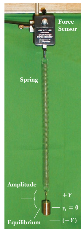
FIGURE 16-11 ■ A common way to measure forces and displacements for a vertical mass–spring oscillator is to hang a light spring with an attached mass from an electronic force sensor. An ultrasonic motion detector can be placed underneath the mass to measure displacements. If we displace the mass vertically from its equilibrium point, it will oscillate between a maximum value of displacement from equilibrium +Y and a minimum value -Y .
