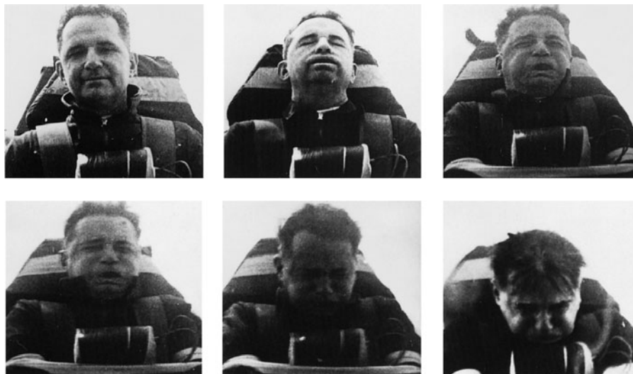
FIGURE 2-13 ■ Colonel J.P. Stapp in a rocket sled as it is brought up to high speed (acceleration out of the page) and then very rapidly braked (acceleration into the page).
