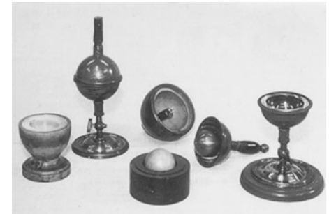
FIGURE 28-16 ■ The simple electrostatic apparatus used by Faraday. An assembled apparatus (second from left) forms a spherical capacitor consisting of a central brass ball and a concentric brass shell. Faraday placed dielectric materials in the space between the ball and the shell.
