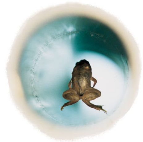
FIGURE 32-20 ■ An overhead view of a diamagnetic frog that is being levitated in a magnetic field. The \vec{B} -field is produced by current in a vertical solenoid below the frog. The solenoid's upward magnetic force on the frog balances the downward gravitational force on the frog. (The frog is not in discomfort; the sensation is like floating in water, which frogs don't seem to mind.)
