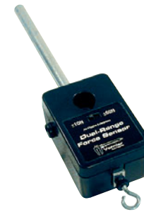
FIGURE 3-8 ■ An electronic force sensor that can be used with a computer data acquisition system. When the hook at the bottom is pushed or pulled, a metal element is compressed or flexed. This is detected by an electronic strain gauge, which puts out a voltage proportional to force.
