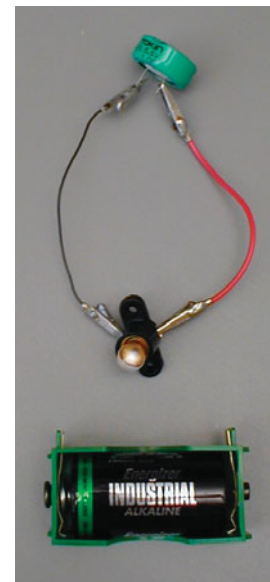
FIGURE 28-4 ■ When a “charged” capacitor is disconnected from its battery and wired in series with a bulb, the energy stored in it can light the bulb for a short period of time.
