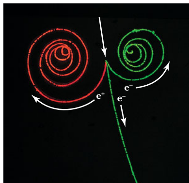
FIGURE 29-5 ■ Color enhanced tracks showing two electrons ( e^- ) and a positron ( e^+ ) in a bubble chamber that is immersed in a uniform magnetic field that is directed out of the plane of the page.
