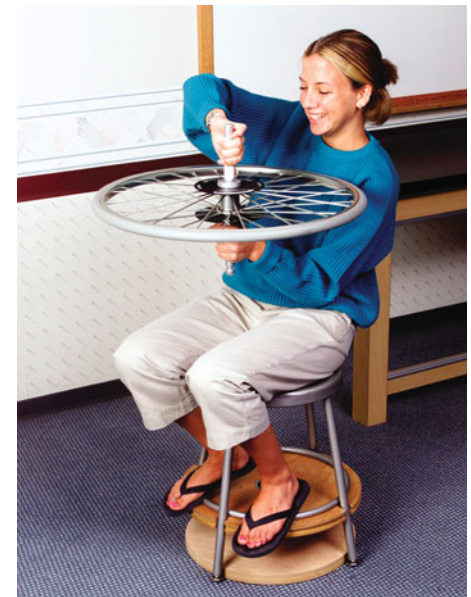
FIGURE 12-2 ■ A student applies a torque to the axis of a rotating bicycle wheel in order to change the direction of the wheel's axis of rotation. (Photo courtesy of PASCO scientific.)
