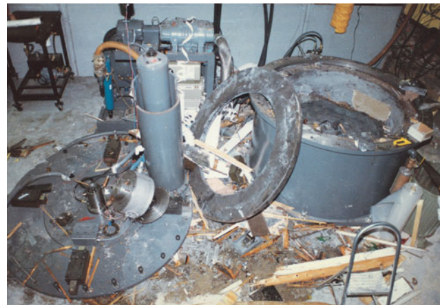
FIGURE 11-16 ■ Some of the destruction caused by the explosion of a rapidly rotating steel disk.
