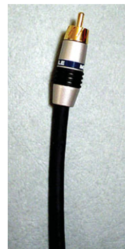
FIGURE 28-11 ■ Coaxial cables and connectors are used for long-distance transmission of television and radio signals. The cable consists of a central conducting wire surrounded by a layer of insulation and then a cylindrical conductor. All three elements are centered on the same axis. Coaxial cables are good examples of cylindrical capacitors.
