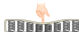
FIGURE P-4 ■ Compressing an innerspring mattress with a force. The mattress exerts an oppositely directed force, with the same magnitude, back on the finger.
