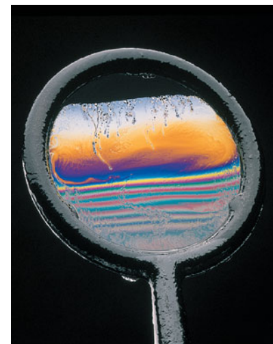
FIGURE 36-14 ■ The reflection of light from a soapy water film spanning a vertical loop. The top portion is so thin that the light reflected there undergoes destructive interference, making that portion dark. Colored interference fringes, or bands, decorate the rest of the film but are marred by circulation of liquid within the film as the liquid is gradually pulled downward by gravitation.
