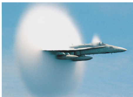
FIGURE 18-27 ■ A cloud formation is produced off the wings of this Navy jet. One plausible explanation is that the cloud forms because of the sudden decrease in air pressure that results as a supersonic shock wave propagates. This causes water vapor in the air to condense.
