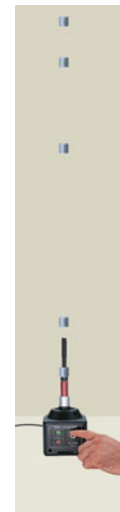
FIGURE 31-16 ■ This demonstration of Lenz's law occurs when an electromagnet is switched on suddenly. The current induced in a metal ring opposes the electromagnet's current. The repulsive forces between the magnet and the ring cause the ring to jump more than a meter. (Photo courtesy of PASCO scientific.)
