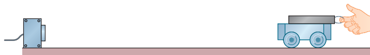
FIGURE 9-15 ■ A variable force is applied to a force sensor attached to a cart on a horizontal track. The cart's position and velocity are recorded using a motion sensor. The friction force is negligible.
