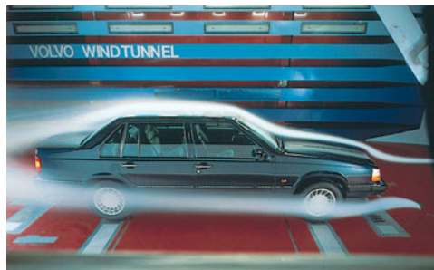
FIGURE 15-21 ■ Smoke reveals streamlines in airflow past a car in a wind-tunnel test.
