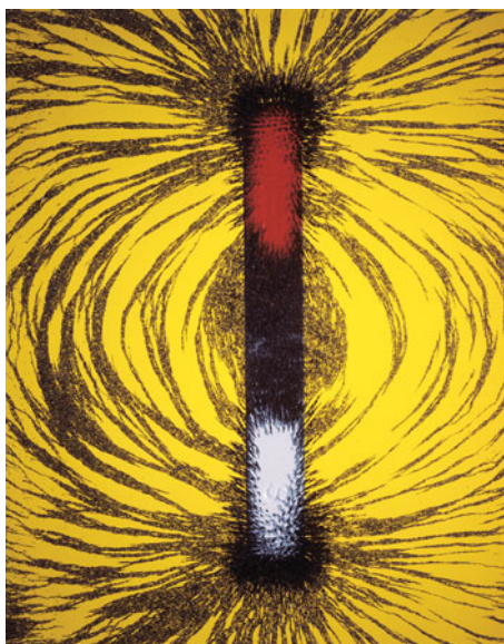
FIGURE 32-13 ■ A bar magnet is a magnetic dipole. The orientations of the iron filings suggest the direction of magnetic field lines.
