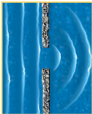
FIGURE 36-4 ■ The diffraction of water waves in a ripple tank. The waves are produced by an oscillating paddle at the left. As they move from left to right, they flare out through an opening in a barrier along the water surface.
