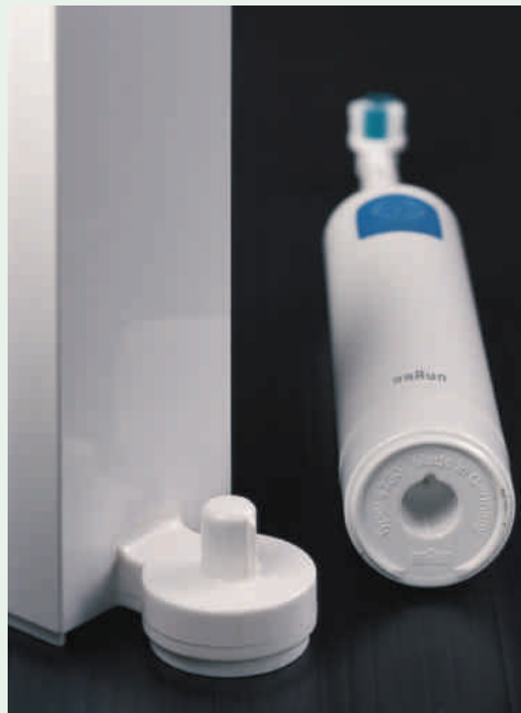
This electric toothbrush uses magnetic induction to charge its battery. The primary coil (coil 1) of N_B turns is in the base unit and the secondary coil (coil 2) of N_H turns is in the handle.
