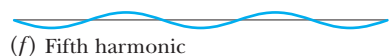
Figure 16-5 The shape of the plucked string (a) is the superposition of the first five harmonics (b–f). Note that the fourth harmonic does not contribute to this particular shape.
