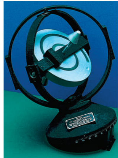
Figure 8-18 A spinning gyroscope maintains its direction in space even when its mount is rotated.
