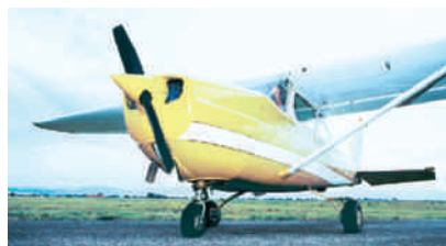
In flight a Cessna 172's propeller blades push the air backward to go forward.
