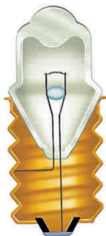
Figure 21-6 Schematic drawing showing the continuous conducting path through a bulb.
