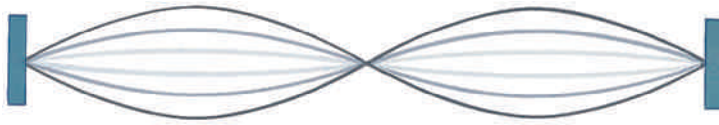
Figure 15-16 A strobe drawing of a standing wave on a rope shows how the shape of the rope changes with time. The shape does not move to the left or right.
