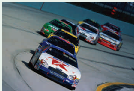
Banking corners allows cars to take curves at high speeds.
