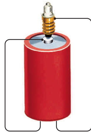
Figure 21-12 When the wire on the left is connected from one end of the battery to the other, producing a short circuit, the light goes out.
