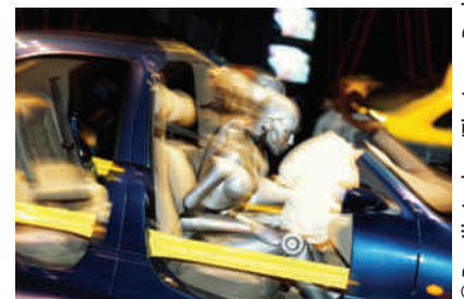
Modern cars employ air bags to protect passengers by increasing their stopping time.
