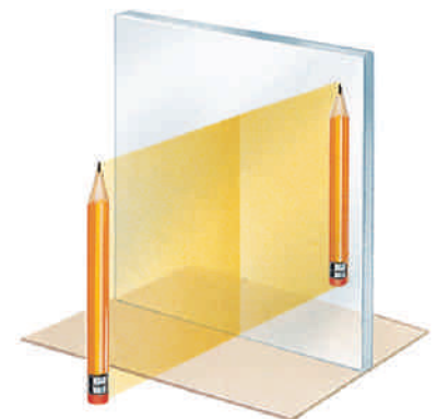
Figure 17-9 The image of a pencil formed by a flat mirror is located behind the mirror.
