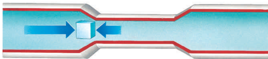
Figure 12-12 The “cube” of fluid entering the narrow region of the pipe must experience a net force to the right.
