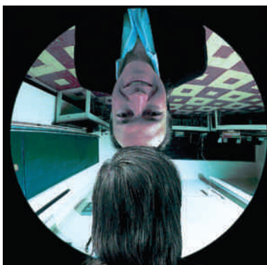
Figure 17-18 An inverted image is formed when the head is located outside the focal point of a concave mirror. Note that both the face and the floor tiles are inverted.
