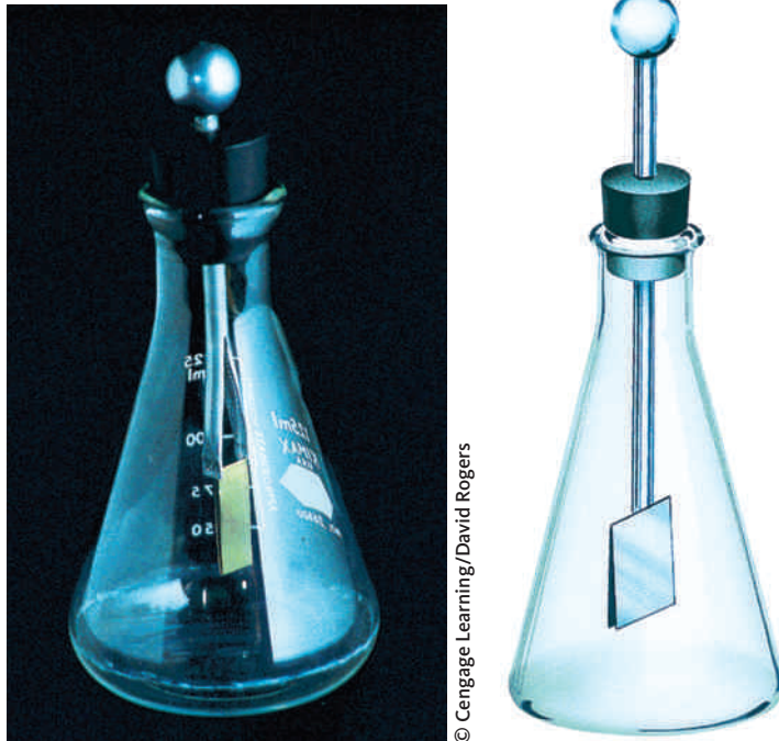
Figure 20-6 An electroscope made from a flask, a metal rod, and two pieces of thin metal foil.
