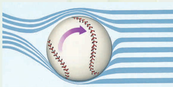
The spinning ball causes the airflow to deflect upward, imparting a downward force on the ball.
