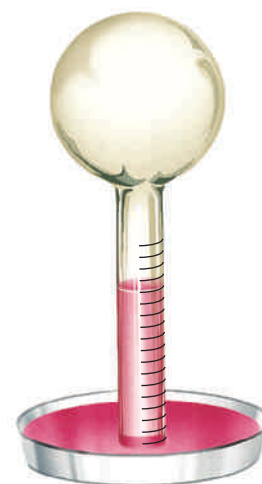
Figure 11-9 The height of the liquid in Galileo's first thermometer indicated changes in temperature.
