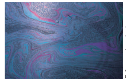
Figure 19-13 The light transmitted through a thin film also displays interference effects.
