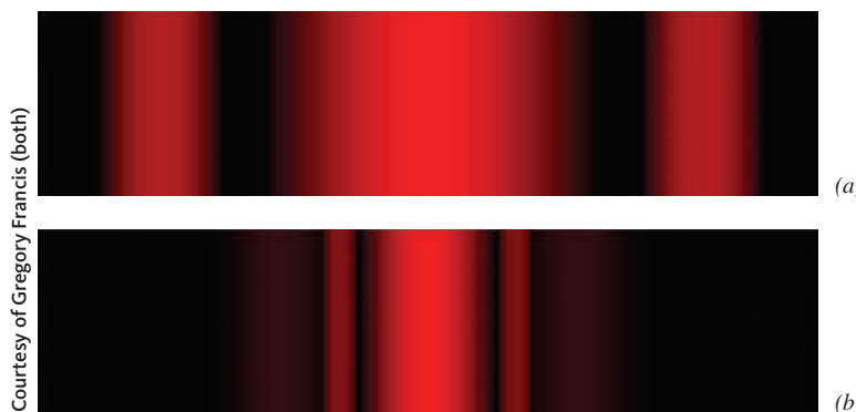
Figure 19-7 Diffraction patterns produced by red light incident on (a) a narrower and (b) a wider slit. The narrower slit produced the wider pattern.
