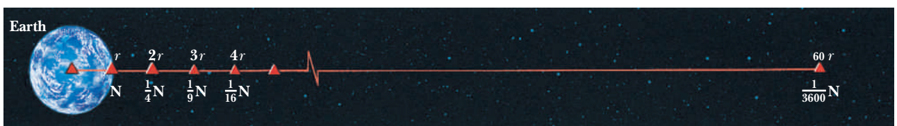
Figure 5-2 The force on a 0.1-kilogram mass at various distances from Earth. Notice that the force decreases as the square of the distance.
