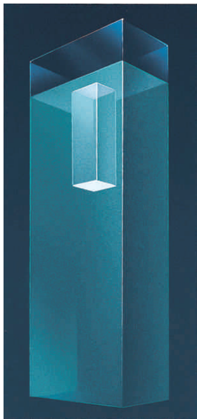
Figure 12-6 The force on the bottom of the box of fluid is equal to the weight of the fluid in the box plus the force of the atmosphere on the top of the box.
