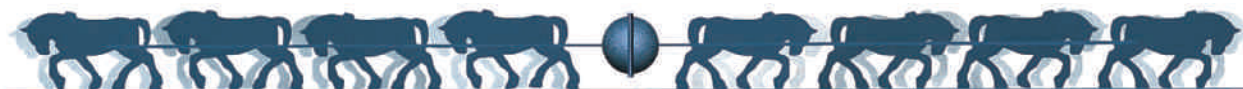
Figure 12-7 Two teams of eight horses could not separate von Guericke's evacuated half spheres.
