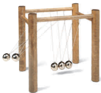
Figure 7-1 The collision-ball apparatus demonstrates the conservation of momentum and kinetic energy.
