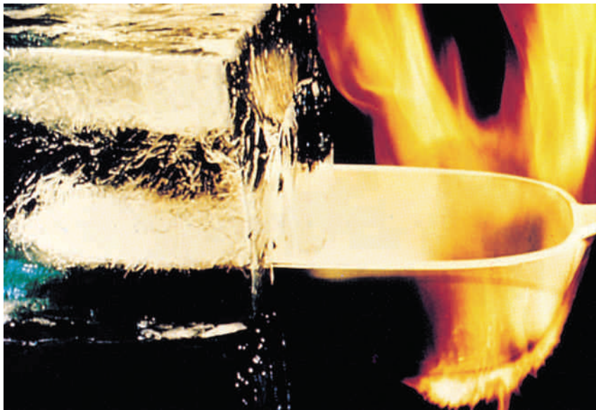
Figure 13-5 The left end of this ceramic dish is ice-cold while the right end is very hot. This occurs because ceramic is a poor conductor of thermal energy.
