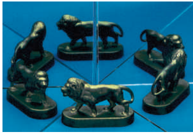
Figure 17-15 When the mirrors form an angle of 60 degrees, five images of the lion are produced.
