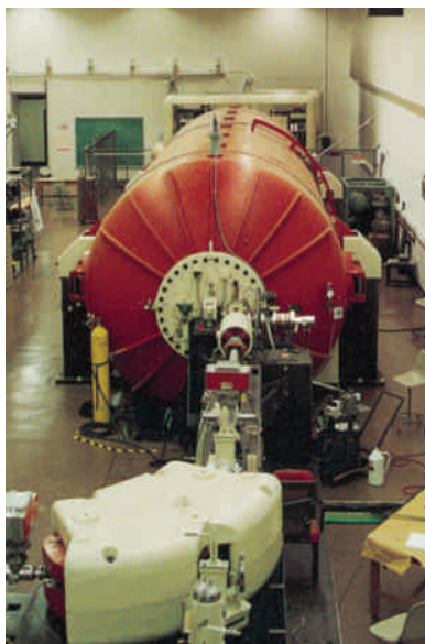
Figure 26-1 This Van de Graaff generator is used to accelerate protons to high velocities to probe the structure of nuclei.
