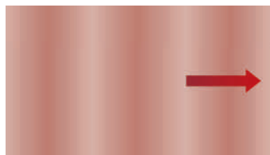
Figure 16-8 A drawing of a longitudinal sound wave. The dark regions represent compressions (high density); the lighter regions represent rarefactions (low density).
