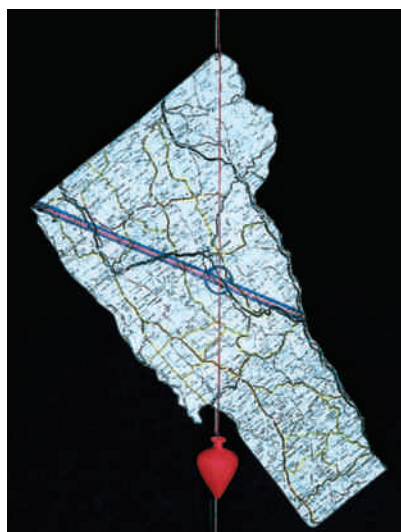
Figure 8-10 The center of mass of the state of Vermont is located by hanging it from two points.
