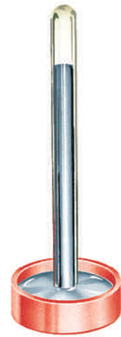
Figure 12-8 In a mercury barometer, the atmospheric pressure is balanced by the pressure due to the weight of the mercury column.
