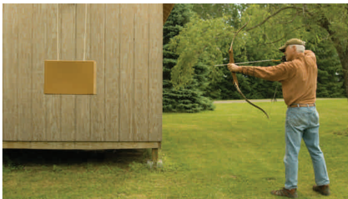
Figure 6-2 Determining the speed of an arrow using conservation of momentum. The momentum of the block and arrow after the collision is equal to the momentum of the arrow before the collision.
