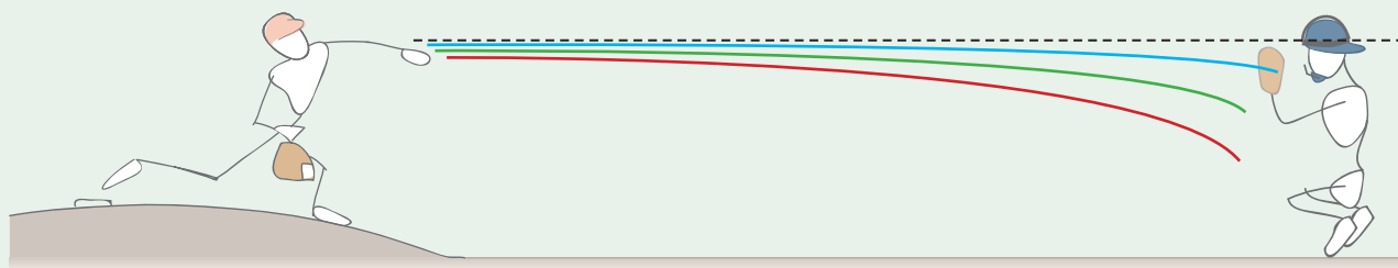
The blue curve represents the ball’s path due to its spin without any gravity. The green curve is the ball’s path due to gravity without spin. The red curve shows the combined effect of spin and gravity.
