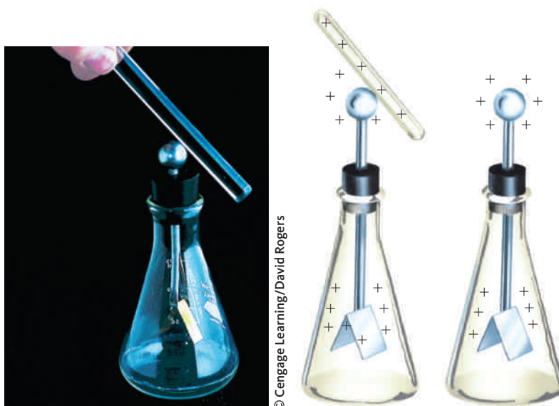
Figure 20-7 When an electroscope is charged by direct contact, it has the same charge as the rod.
