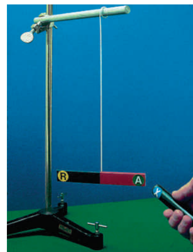
Figure 22-1 Magnetic poles can be identified by their attraction to and repulsion by known poles.
