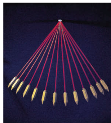
A strobe photograph of a pendulum taken at 20 flashes per second. Note that the pendulum bob moves the fastest at the bottom of the swing.
