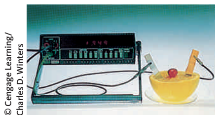
A modern version of Volta's demonstration that zinc and copper rods inserted into a grapefruit produce a potential difference. (The cherry is for decorative purposes only.)
