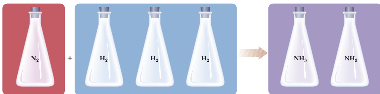
Figure 11-3 Gases combine completely to form compounds when the ratios of their volumes are equal to the ratios of small whole numbers. One liter of nitrogen combines completely with 3 liters of hydrogen to form 2 liters of ammonia.
