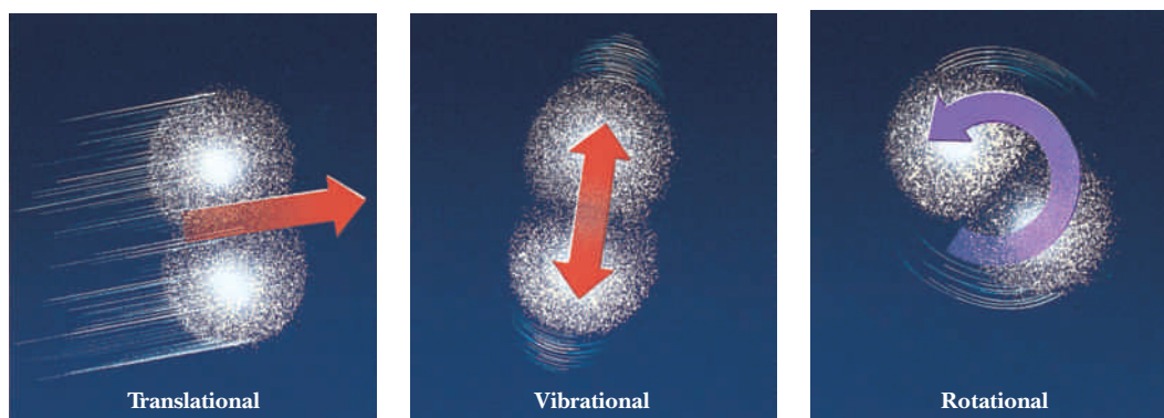
Figure 13-3 Three forms of internal energy for a diatomic molecule.
