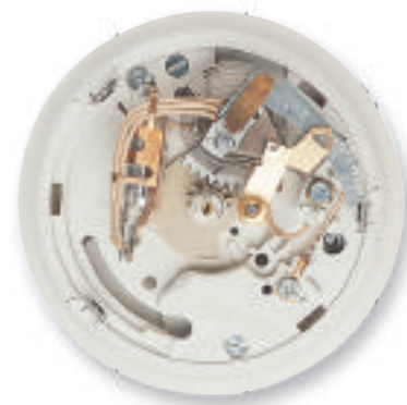
■ Figure 13-22 In this thermostat, a coiled bimetallic strip controls the flow of mercury for opening and closing electrical switches.
