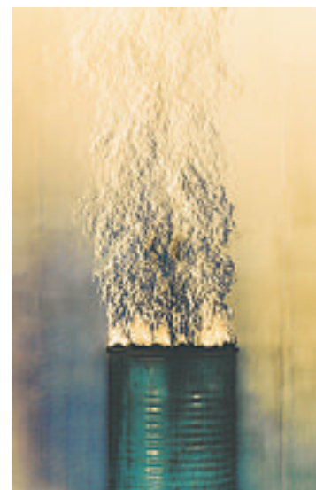
■ Figure 13-5 This image was made by a special technique that enables you to see different densities in the air. Convection currents are set up as warmer, less dense air rises and cooler, denser air sinks.
