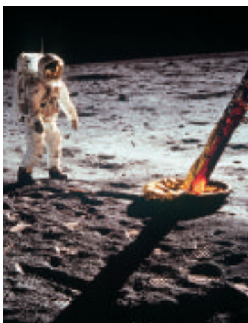
■ Figure 13-2 The astronaut and the landing module both exert pressure on the lunar surface. If the lunar module had a mass of approximately 7300 kg and rested on four pads that were each 91 cm in diameter, what pressure did it exert on the Moon's surface? How could you estimate the pressure exerted by the astronaut?
