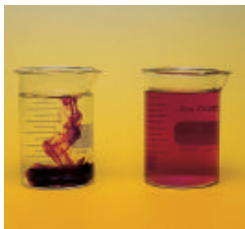
■ Figure 12-15 The spontaneous mixing of the food coloring and water is an example of the second law of thermodynamics.
