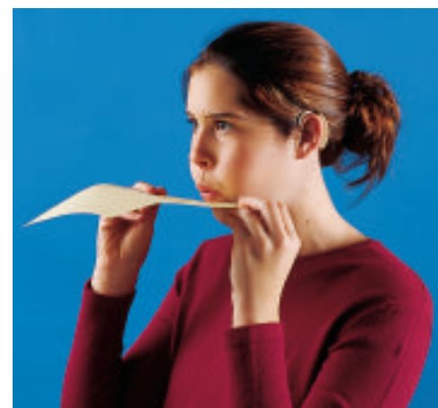
■ Figure 13-15 Blowing across the surface of a sheet of paper demonstrates Bernoulli's principle.
