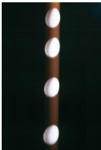
■ Figure 3-14 An egg accelerates at 9.80 \text{ m/s}^2 in free fall. If the upward direction is chosen as positive, then both the velocity and the acceleration of this egg in free fall are negative.
