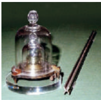
■ Figure 1-3 The standards for the kilogram and meter are shown. The International Prototype Meter originally was measured as the distance between two marks on a platinum-iridium bar, but as methods of measuring time became more precise than those for measuring length, the meter came to be defined as the distance traveled by light in a vacuum in 1/299\,792\,458 s.
