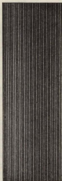
FIG. 29.6 Fresnel's biprism interference bands (magnified).
