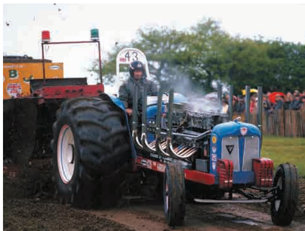
Figure 1.5 In a tractor pull, vehicles develop up to 9000 horsepower to accelerate a sled, until they can no longer overcome the constantly increasing frictional forces. Dragsters, on the other hand, accelerate right up to the finish line.
