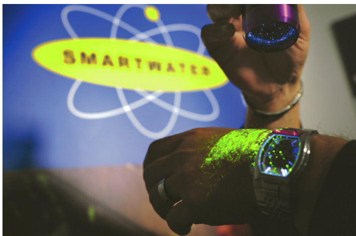
Figure 3.7 This man has been sprayed with 'smartwater'. Each batch of the water has a special DNA, which determines where a material has come from. The 'smartwater' shows up under UV light. Such materials are now widely used to mark property.
