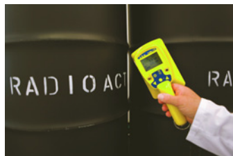
Figure 4.5 This geiger counter is being used to determine the activity of radioactive waste which is stored underground.
