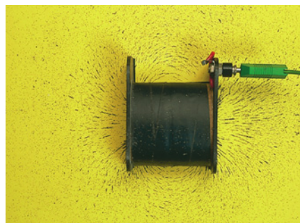
Figure 2.8 The iron filings show the shape of the magnetic field around a solenoid.
