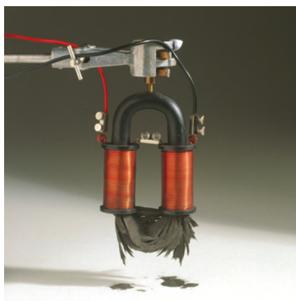
Figure 3.7 This photograph shows the design of a practical laboratory electromagnet. It is made strong by two coils with many turns of wire to increase the magnetising effect of the current. When the current is switched off the iron filings will fall off the magnet.
