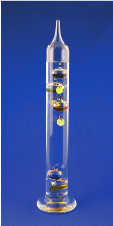
Figure 1.3 Galileo's thermometer (see Study Question 2).
