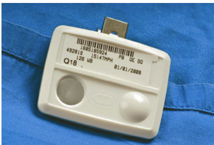
Figure 5.2 To check the amount of radiation that workers in a nuclear power station are exposed to, they wear special radiation-sensitive badges, like the ones in this photograph. At the end of each month the sensitive film in the badges is developed and examined.
