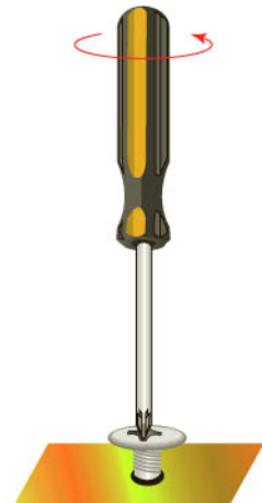
Figure 11.4 A screwdriver is used to insert a screw – a broad handle allows us a good grip and leverage.
