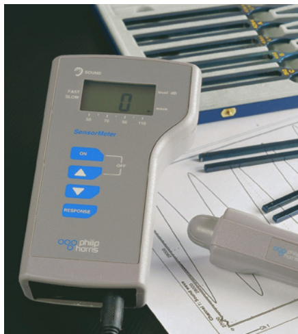
Figure 10.3 This data logger can be used to record the waveforms produced by different instruments.
