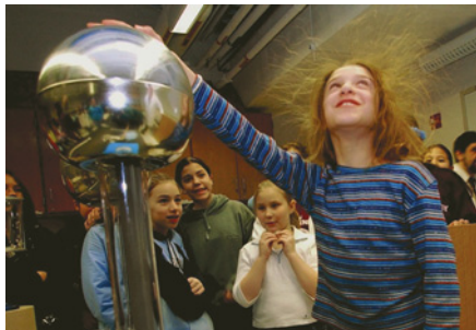
Figure 9.1 Using a Van de Graaff generator to demonstrate that like charges repel each other.
