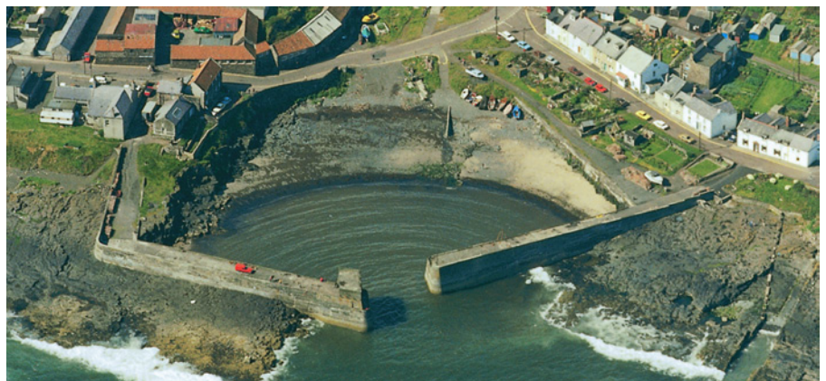
Figure 2.7 In this photograph you can see water waves diffracting as they pass through a harbour entrance. Water waves have a large wavelength, and so they spread out a lot when they diffract through such a gap.
