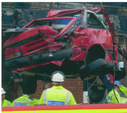
Figure 2.3 This car has been in a major accident. A fast moving, massive object like a car experiences a very large force when it decelerates rapidly. The force is large enough to crumple the roof.
