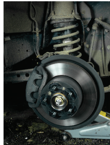
Figure 3.22 The springs used in car suspension systems need to have a high spring constant.
