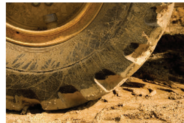
Figure 6.2 The area over which the force is acting affects the pressure it exerts.
