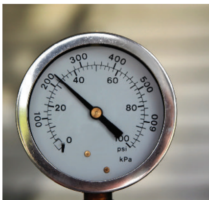
Figure 6.37 Pressure gauges may read absolute pressure or gauge pressure.
