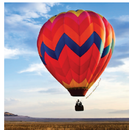
Figure 6.47 The buoyant force from the air keeps the hot balloon in the air.
