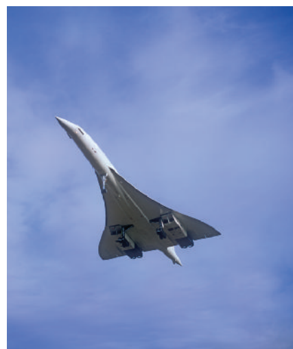
Figure 7.18 When Concorde flew at over twice the speed of sound, it got so hot that it increased its 61.6\text{ m} length by about 30\text{ cm} .
